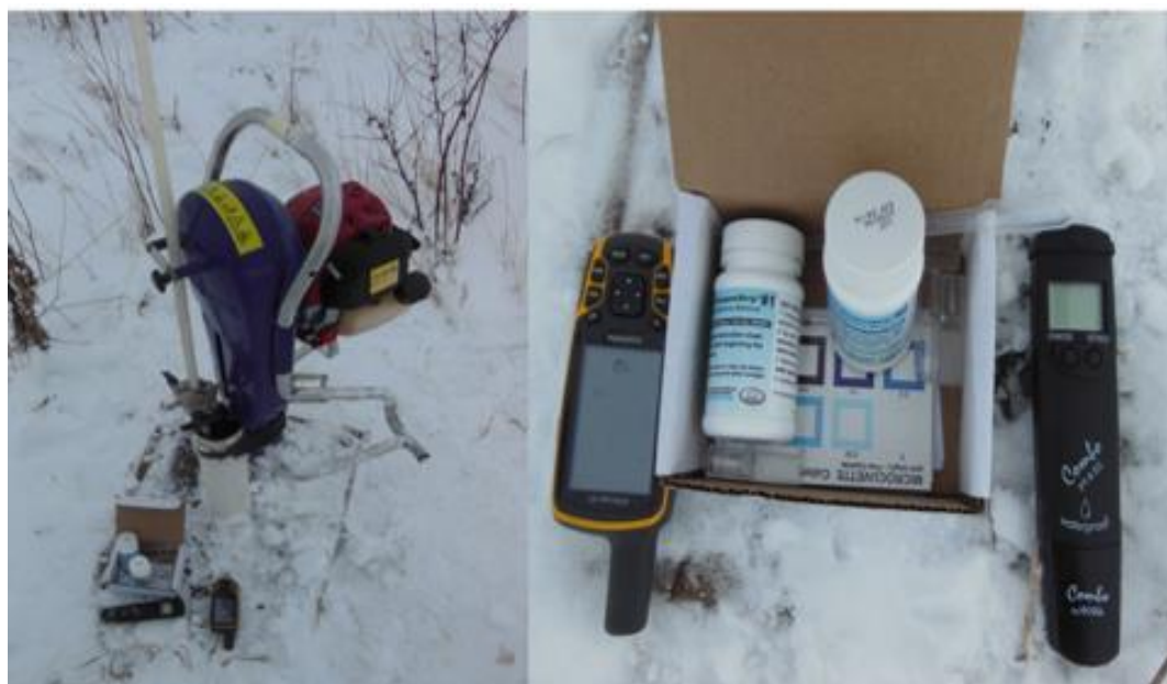
Fig. 4. Water analysis equipment. Ph/EC/TDS/Temperature meter and Cyanide test kit.
