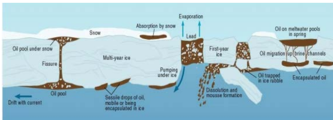
Figure 1. Behaviour of oil in or beneath ice and snow [2]
