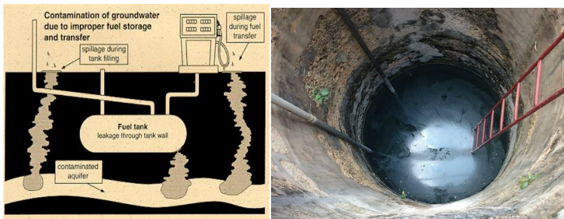
Pic. 2. Cause of underground oil spill and its effect on a well [6, 7]
