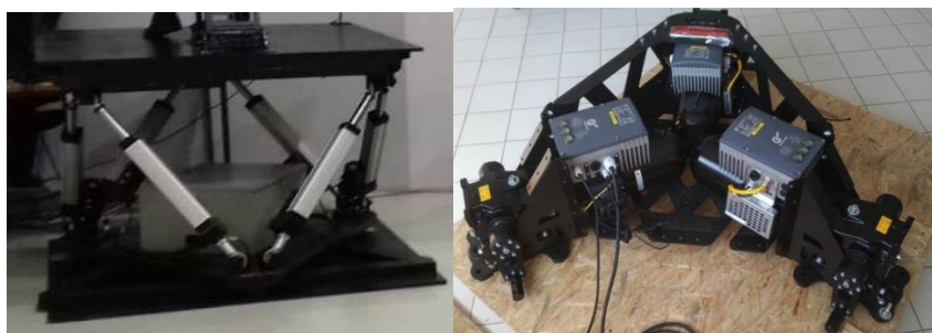
Figure 2. Compact dynamic platforms (hexapod on the left, tripod on the right-side image)
