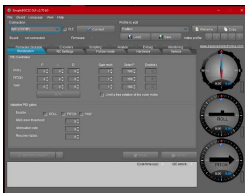
Fig. 3. Adaptation and PID tuning of selected stabilization system via Basecam GUI
